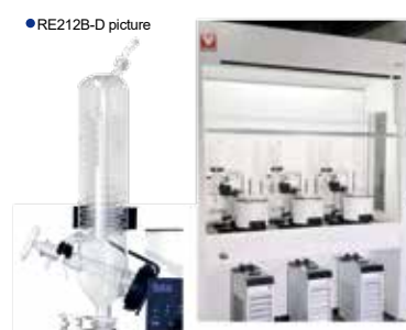
In the fume hood, set up 3 vertical glass sets.
