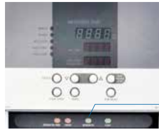
Water level monitoring, refrigeration unit monitoring, refrigeration unit action indicator
