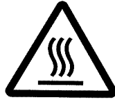
Danger! High temperature
