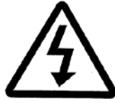
Danger!: High voltage
