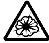
Danger!: Hazard of explosion
