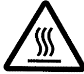
Danger!: High temperature
