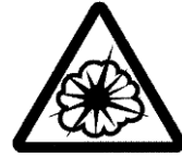
Danger!: Hazard of explosion
